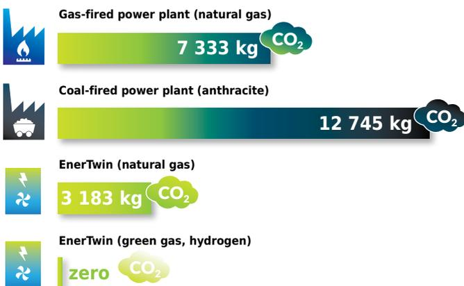
When generating this same amount of electricity in 5000 running hours, an EnerTwin can reduce CO<sub>2</sub> emissions by more than 9.5 tons compared to a coal-fired power plant! These reductions are even further improved when using green gas or biomethane.
